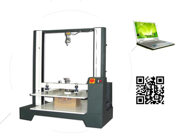
**Applications**: PT-8216 Computer System Container Compression Tester shall be used for testing resistance about all kinds of packaging body and cartons, the result would be regarded as the important references of the height of piling up the cartons and design the cartons.
